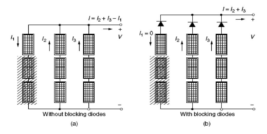
Blocking diodes prevent reverse current from flowing down malfunctioning or shaded strings.
