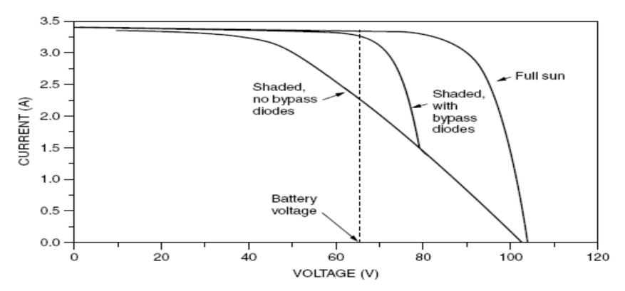
Impact of bypass diodes. Drawn for five modules in series delivering 65 V to a battery bank. With one module having two shaded cells, charging current drops by almost one-third when there are no bypass diodes. With the module bypass diodes there is very little drop.
