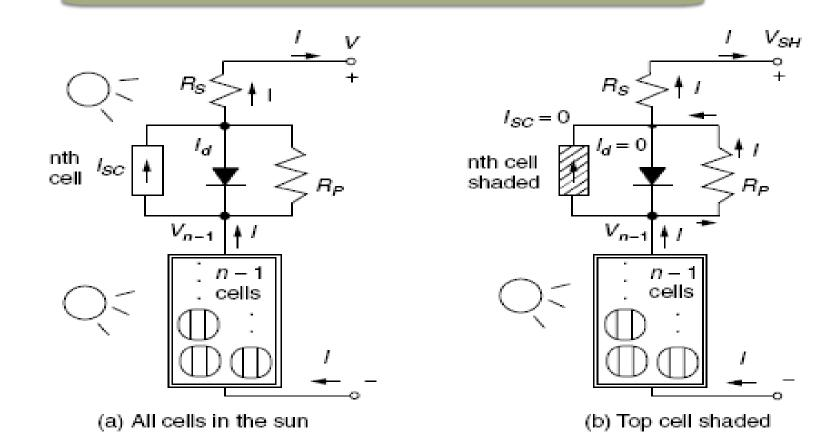
A module with *n* cells in which the top cell is in the sun (a) or in the shade (b).
